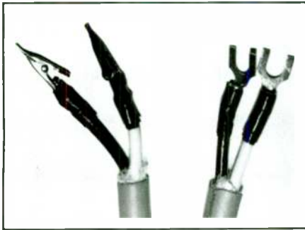
PHOTO 3: Monster Cable power line 2 is used for internal and external wiring for the woofers. The solid copper alligator clips allow the driver-coupler to be removed with a twist-and-pull motion. The Old Colony spade lugs terminate to Old Colony five-way binding posts on the PVC pipe.
