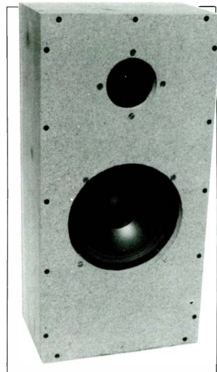
PHOTO 2: 1 cubic foot closed-box enclosure using Radio Shack's 40-1021 8" driver.
