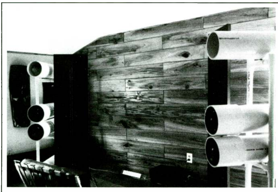
PHOTO 8: "Near-field" listening position with ears about 0.9 meters from the ribbons, while the woofers are about 1.5m from the side walls. Note the lack of oak trim. I spent about seven months listening in this position.
