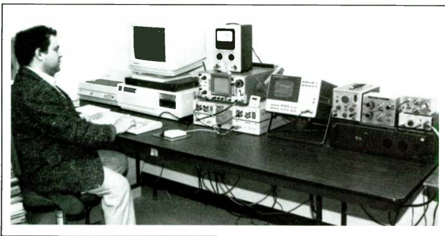
PHOTO 10: Ken Kantor's driver test setup, including a PC/AT control computer, an Audio Precision system, and an HP FFT analyzer.
