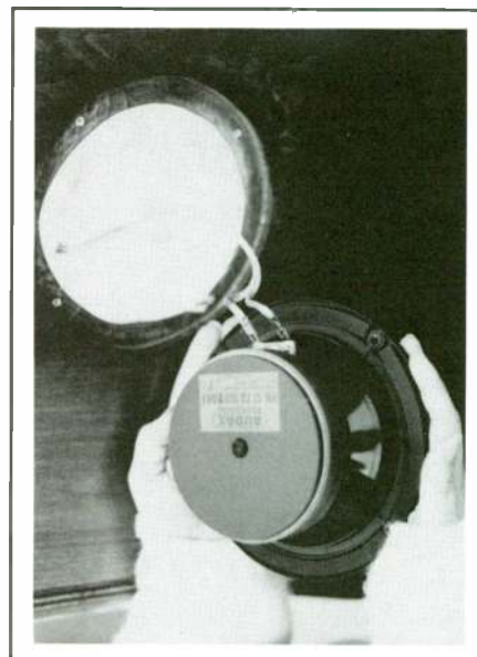
PHOTO 2: The PR17TX100 driver about to be inserted into the speaker.
