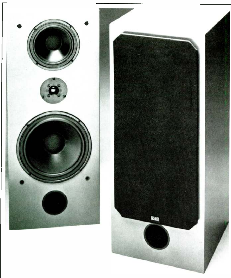
PHOTO 8: The Model 100, a vented studio monitor, features an angled back panel for proper listening orientation. The top mounted midrange has a crossover point at 150Hz and its own sealed enclosure.
