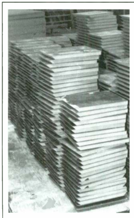
PHOTO 4: Precut MDF boards with bonded laminate surfaces awaiting assembly.
