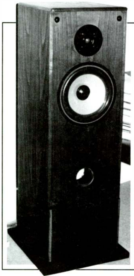
PHOTO 1: The completed first "final" enclosure. The lower front panel indicates the approximate extent of the lower compartment housing the crossover filters.
