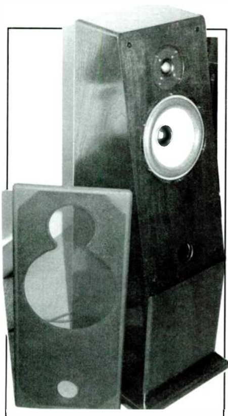
PHOTO 2: The completed final enclosure. The lower compartment housing the crossover filters is approximately 100 mm high.
