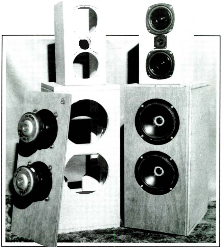
PHOTO 1: Original test system with its minimum-cost mid-high module, now replaced with multi-directional, eight-driver (per side) unit. The woofer itself was inverted to make use of the Allison effect, and the side panels were modified by attaching extra half-inch-thick plywood panels to the outside surfaces.
