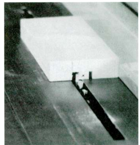
PHOTO 8: Cleaning out the center of a groove.
