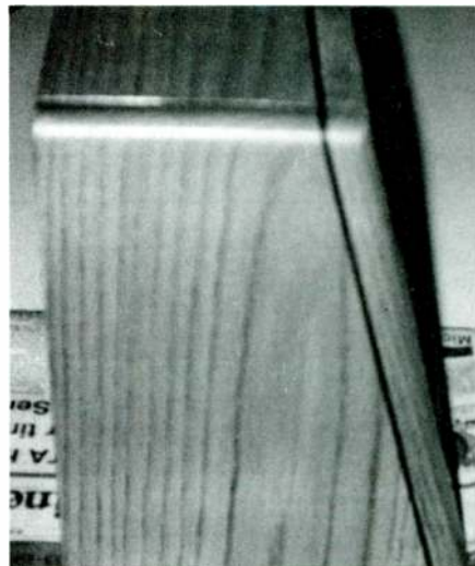
PHOTO 3: A groove improves the appearance of the joints.
