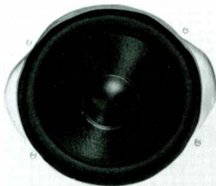
PHOTO 17: Completed Vifa subwoofer ready to be installed. Both holes were enlarged to ensure the rubber surround would not contact the plywood during large excursions.
