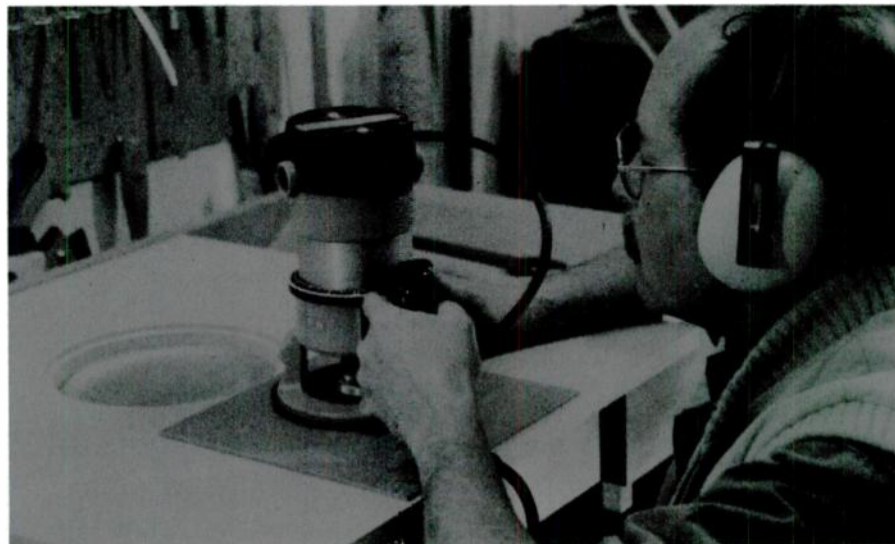
PHOTO 9: Moving the router around until the entire surface of the hole has been covered.
