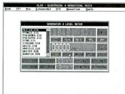
FIGURE 2: The Generator and Level Meter control panel.
