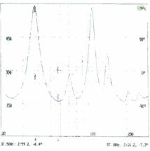
FIGURE 48: ZIN for dual drivers X in series with rubber throat and full <sup>3</sup>/<sub>4</sub>L extension.
