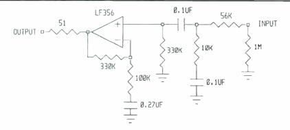
FIGURE 39: Schematic for active waveguide equalizer.
