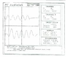
**FIGURE 5:** PC AudioLab oscilloscope measurement of the speed of sound in stuffed transmission line.
