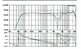
CALSOD 3.000 response of a two-way system calculated for the on-axis design case, as well as +/-15° above and below the principal listening axis.
