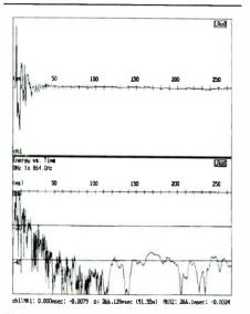
FIGURE 36: Energy-time curve for dual drivers X on original waveguide.
