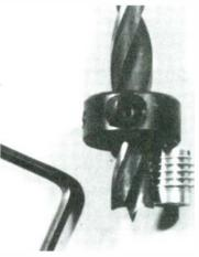
**PHOTO 10**: Setting the depth of a drill stop for an insert.
