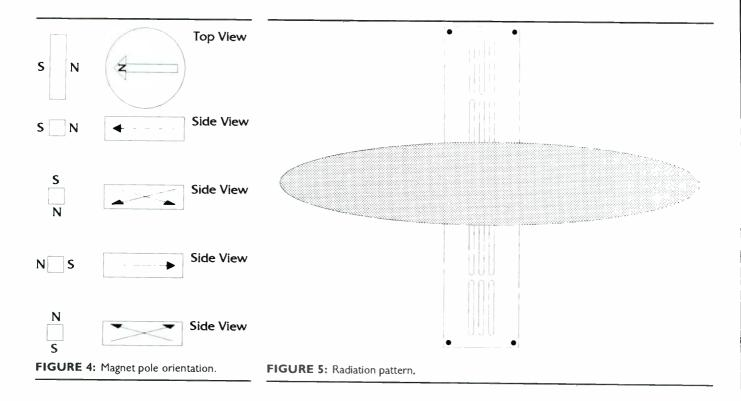
$2-30\Omega$ . Given the tweeter crossover formula:  $F = 1/(2 \times 3.14 \times C \times Z)$ , the crossover point will change, which will also affect the speaker's radiation pattern. This planar speaker allows the single crossover point to be below 300Hz.
