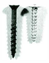
**PHOTO I**: Two common screws: on the left is a common flathead, with threads starting about one-third of the way down the shank; on the right is a roundhead, with tapping threads the full length of the shank.
