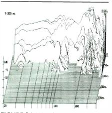
**FIGURE 34:** Waterfall plot for dual drivers X with rubber throat, stiffened full <sup>3</sup>/<sub>4</sub>L extension.
