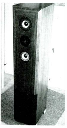
**PHOTO 8:** Completed TL enclosure without base attached.
