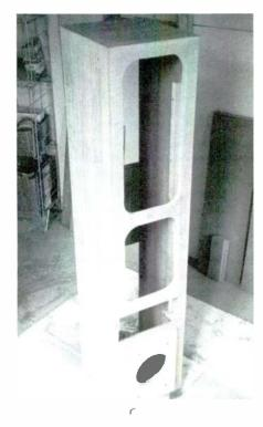
**PHOTO 4:** Assembled main TL cabinet without rear panel attached.
