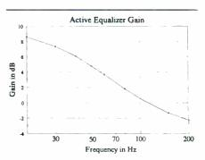
**FIGURE 40:** Measured response of active equalizer.
