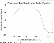
**FIGURE 41:** Pink-noise test results for waveguide with active equalizer and active crossover.
