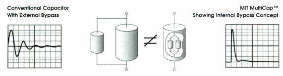
Multiple resonances in a 2  $\mu f$  capacitor bypassed with an external .22  $\mu f$  capacitor. Result: high distortion.
