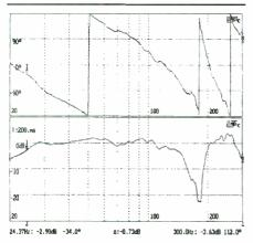
FIGURE 42: Near-field response dual drivers X, rubber throat, full <sup>3</sup>/<sub>4</sub>L extension, and active equalizer.
