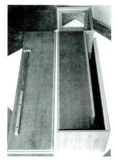
**PHOTO 5:** Cut-away view of middle-section divider in place.
