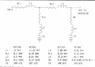
FIGURE 45: Schematic for passive crossover/equalizer.
