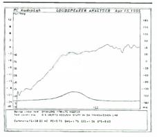
FIGURE 8: PC AudioLab impedance and SPL measurement for 0.5 lb/ft<sup>3</sup> stuffing.
