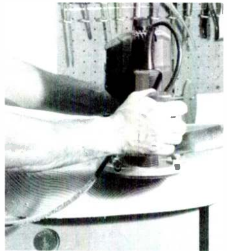
PHOTO 12: Using a router with a roundover bit to smooth the edge of the base.
