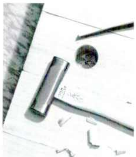
PHOTO 7: A specially designed Japanese chisel for cleaning out holes. Note the small hammer that is made for use with Japanese chisels. One face is flat and the other is slightly rounded.
