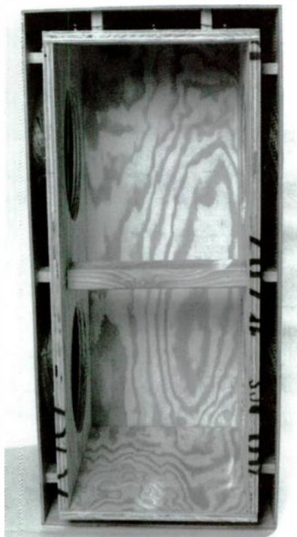
PHOTO 8: Front view of completed box prior to pouring cement.
