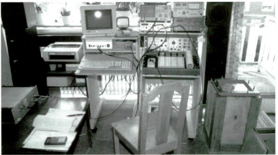
PHOTO 3: Test setup for vibration measurements.
