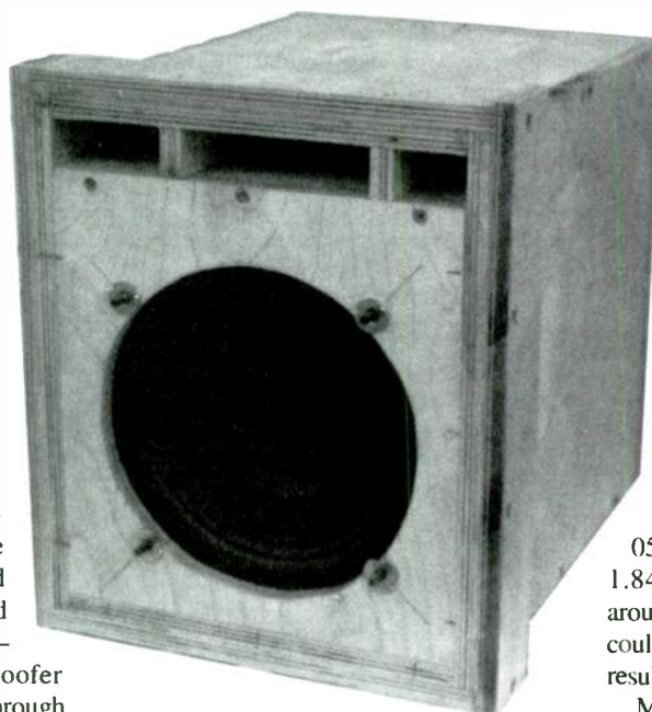
PHOTO 1: The completed reflex box.
