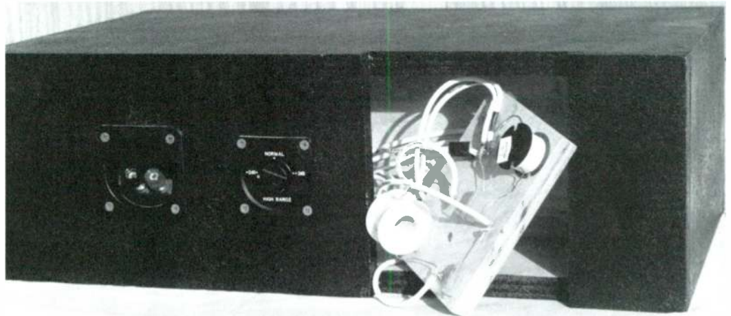
PHOTO 1: Crossover in the open back of the enclosure.
