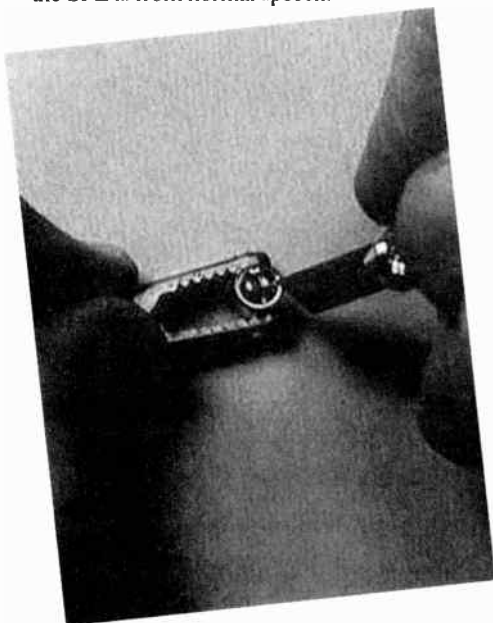
PHOTO 4: Cutting modification on the WM-060AY capsule.
