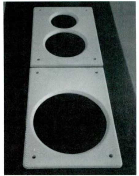
PHOTO 13: Grille boards, shaped and primed.
