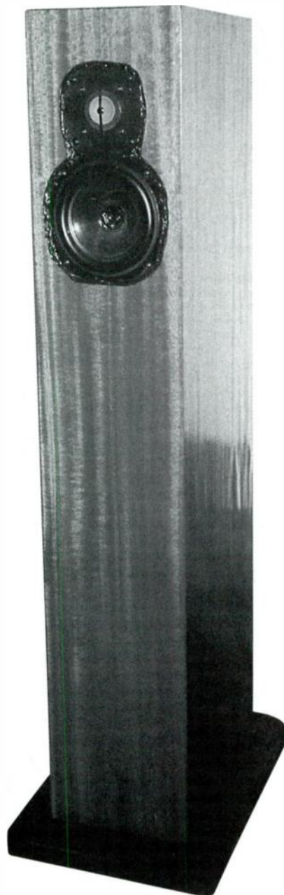
PHOTO 1: Finished speaker, showing rib-bon-stripe mahogany veneer and spiked base.
