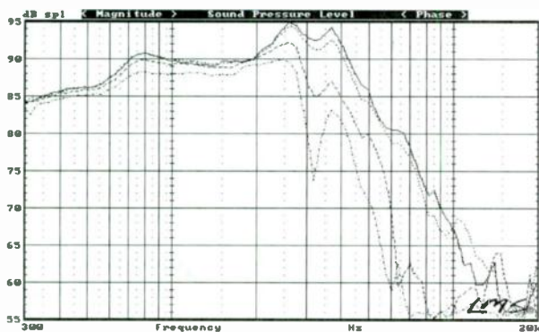
FIGURE 5: 18W/8545K on- and off-axis frequency response (solid = 0°, dot = 15°, dash = 30°, dash/dot = 45°).
