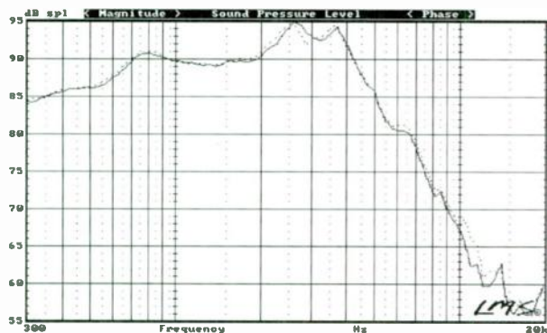
FIGURE 6: 18W/8545K SPL comparison for two samples.
