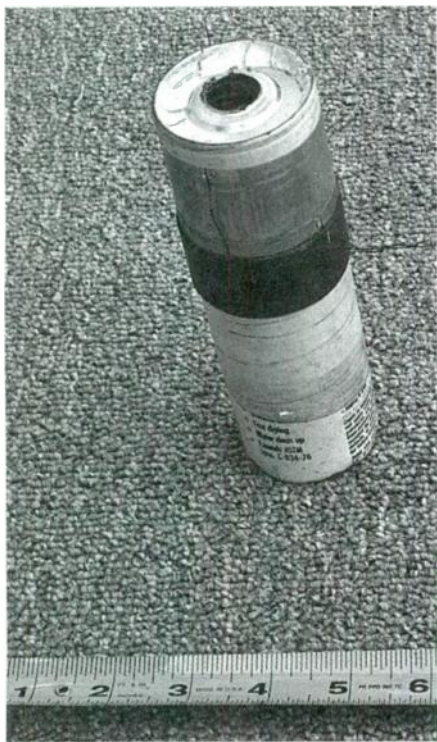
PHOTO 8: Modified motor coil on aluminum former mounted on caulk-tube fixture, ready to be glued to the cone. The blackened wire throws off heat better, helping out marginally with power handling.
