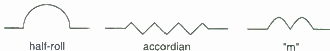
FIGURE 2: Three different surround profiles. (Reprinted from Richard Honeycutt's "Loudspeaker University," VC October 1995, p. 27.)
