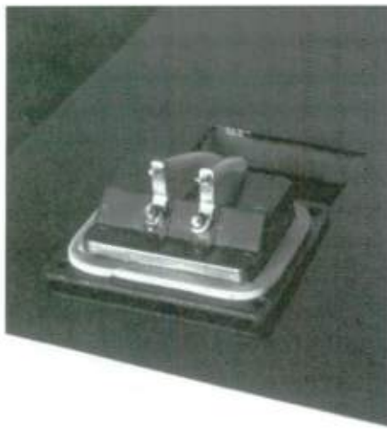
PHOTO 8: Input cup. Add foam gasket material before installing (I used 1/8" x 1/4" foam weather stripping, because I wasn't sure if there was enough gasket material supplied with the kit).
