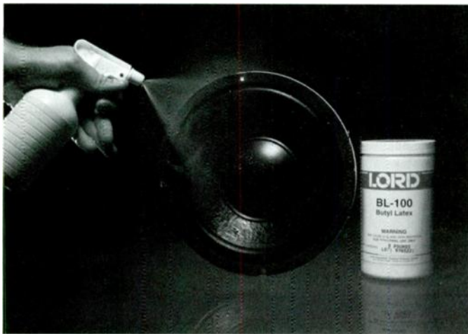
PHOTO 2: This metal cone is being treated with Lord Corporation's BL-100.
