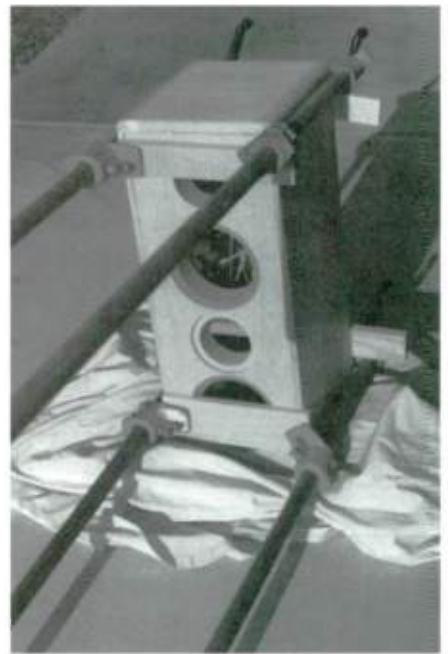
PHOTO 10: Front baffle glued and clamped.
