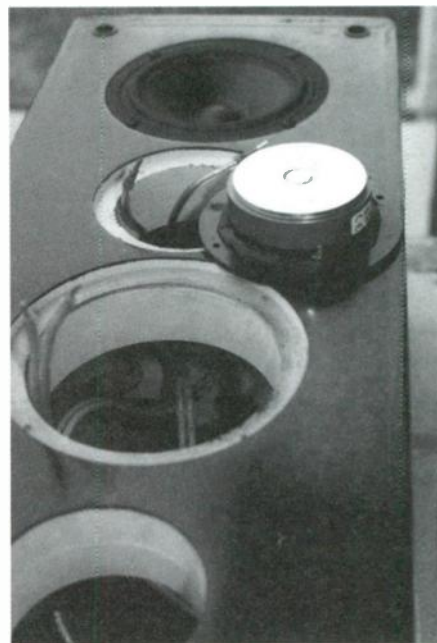
PHOTO 7: Gasket material on driver ready to mount.
