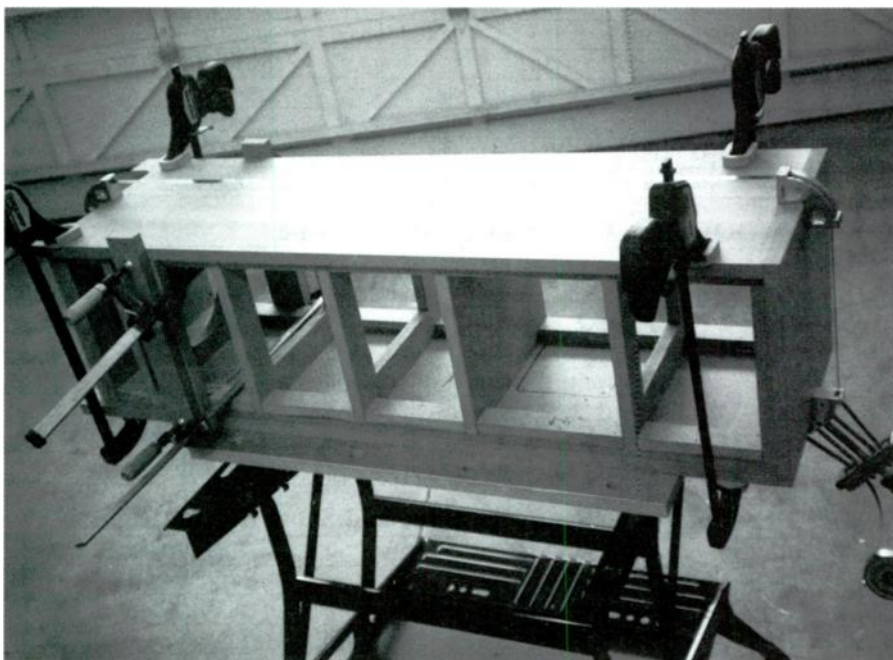
PHOTO 9: Clamped side panels.
