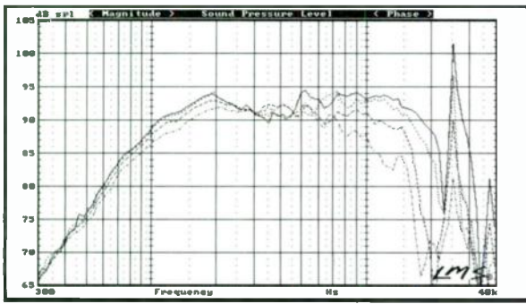
FIGURE 5: 27TAF/G tweeter on- and off-axis frequency response (solid = 0°, dot = 15°, dash = 30°, dot/dash = 45°).
