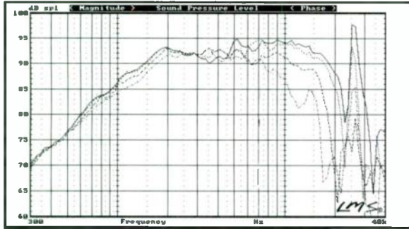
FIGURE 6: 27TAF/G tweeter on- and off-axis frequency response (solid = 0°, dot = 15°, dash = 30°, dot/dash = 45°).
