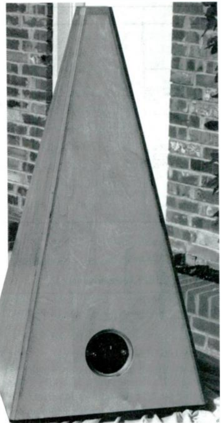
PHOTO 3: Back of speaker, showing recessed treble control and terminals.
