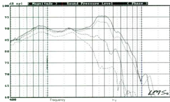
FIGURE 5: On- and off-axis frequency-response curves (solid = 0°, dot = 15°, dash = 30°, dash/dot = 45°).
