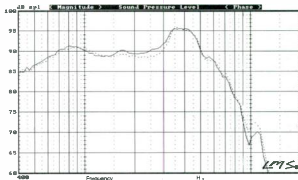
FIGURE 6: 18W/8546 two-sample SPL comparison.
