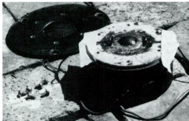
PHOTO 13: Treble dome with mounting flange removed.
