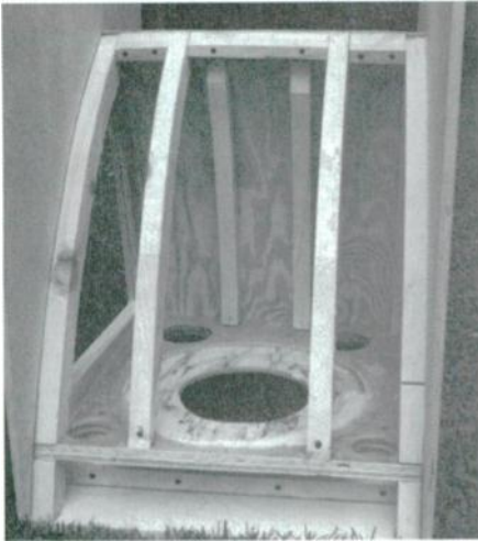
PHOTO 7: Rear horn panel installed; note offset of braces to clear driver frame.
