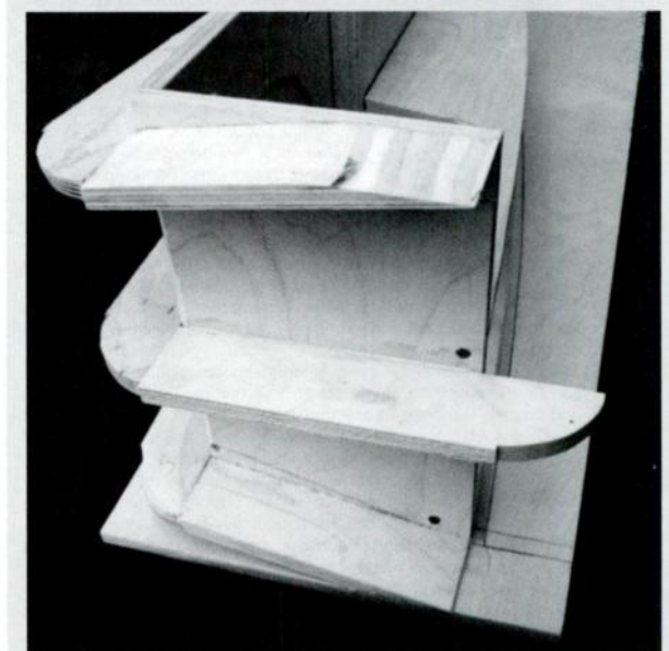
PHOTOS 5 AND 6: Construction adhesive filling the reflectors' joints.
