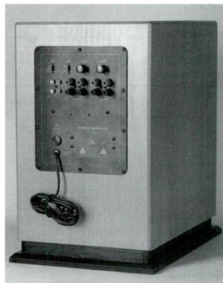
PHOTO 3: The airtight DT105 subwoofer module fits into a rectangular cutout in the enclosure back.
