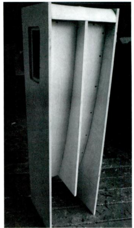
PHOTO 9: The curved reflector attached with hot-melt glue.
