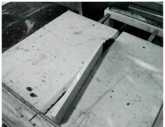
PHOTO 4: Cutting a plate reflector's ends.
