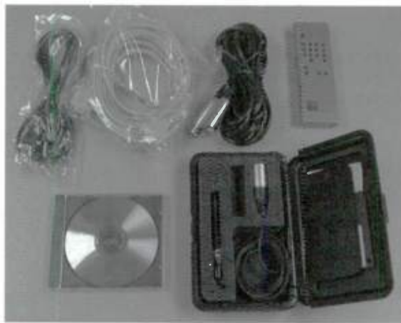
PHOTO 3: TACT RCS 2.2 accessories. Top row: power cable, RS-232 (9-pin) data cable, mike cable, remote control; bottom row: software CD, calibrated microphone with calibration file disk.
