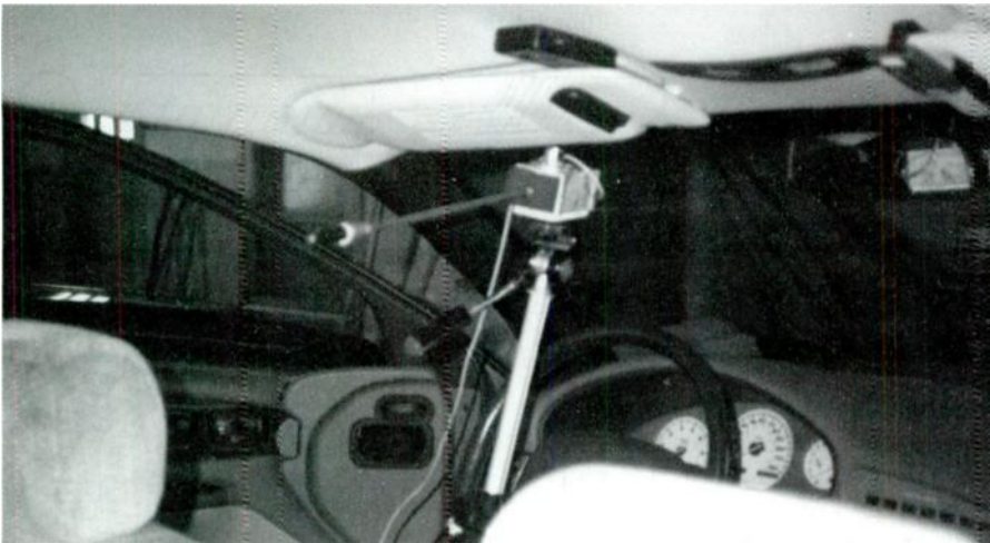
PHOTO 7: Panasonic WM-60AY capsule (used in Mitey Mike II) at driver's ear location.
