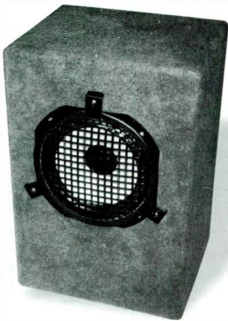
PHOTO 1: Focal 8K5412 in 0.9ft 3 sealed box.
