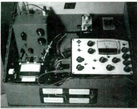
PHOTO 5: Low-distortion sine/cosine sweep oscillator, true-RMS detector, audio filter, and mike preamp.
