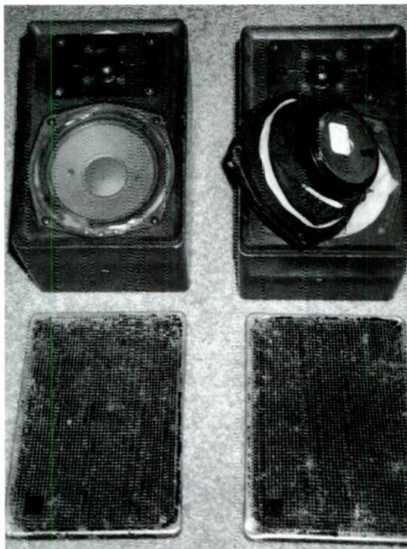
PHOTO 3: Felt damping on a/d/s 5" mid/woofer.
