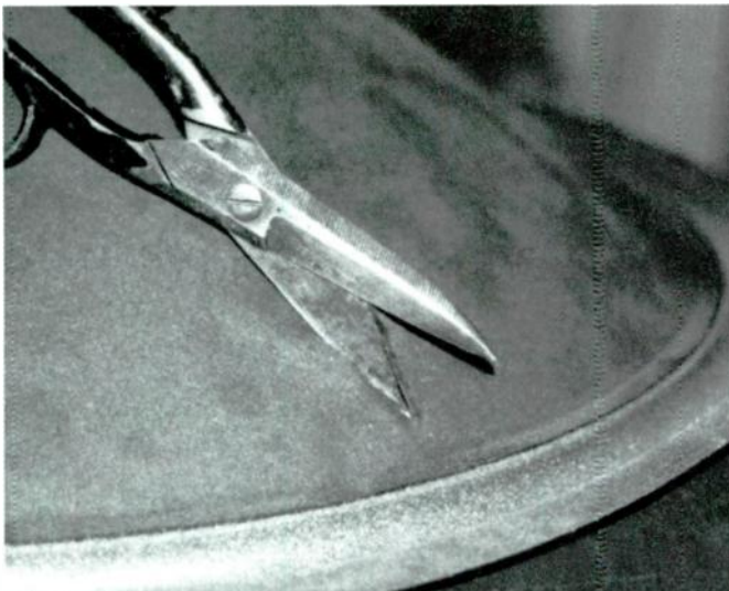
PHOTO 20: Cone is cut away from flat diaphragm.
