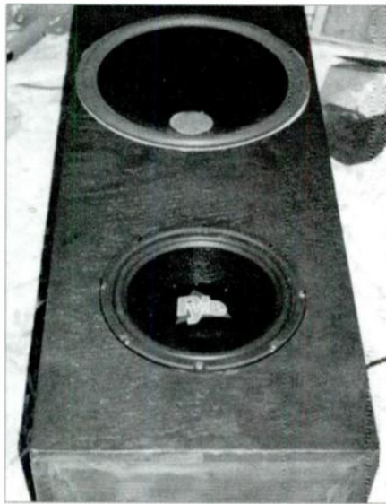
PHOTO 11: Finished enclosure showing a passive instead of a port.
