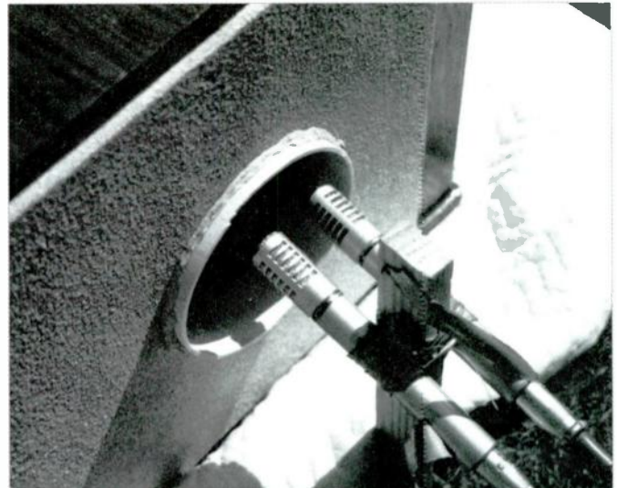
PHOTO 22: Mike is in position to be equalized.
