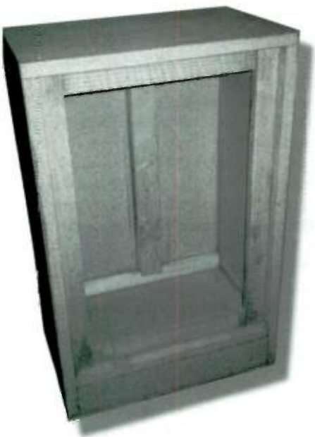
PHOTO 4: Completed cabinet without front panel. The inside bracing is red oak, which gives good holding power for the screws.
