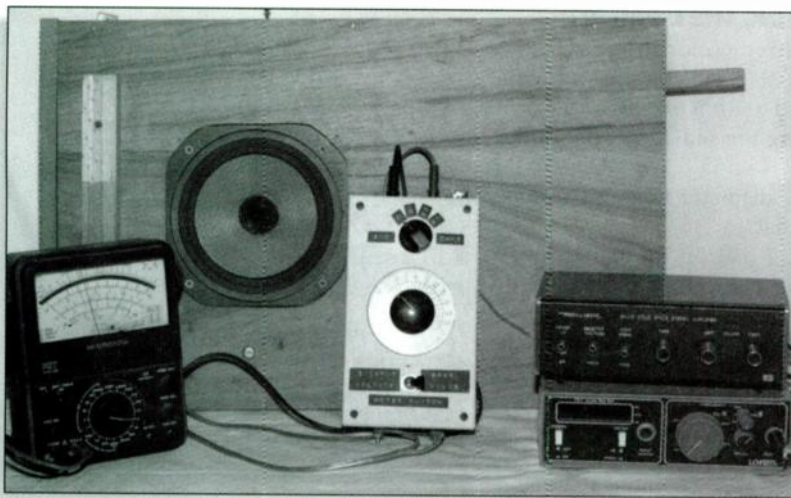
PHOTO 3: Device being used to measure impedance of a driver mounted in a test box.
