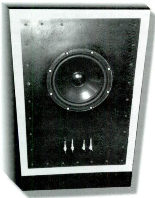
PHOTO 1: The completed enclosure. The oak frame was ebony-stained after this photo.
