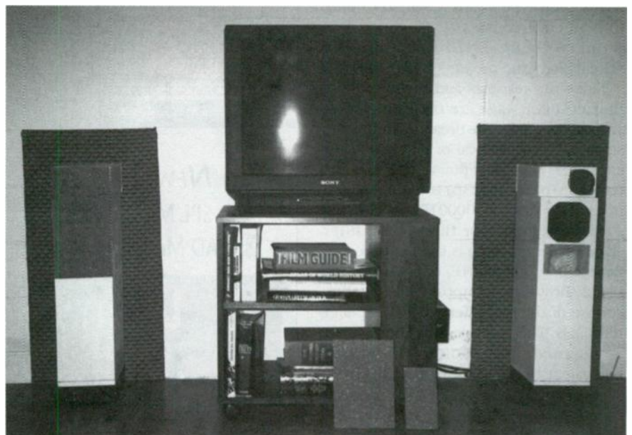
PHOTO 1: The completed speakers set alongside the TV receiver. At this distance there is no effect of the unshielded drivers on the display.
