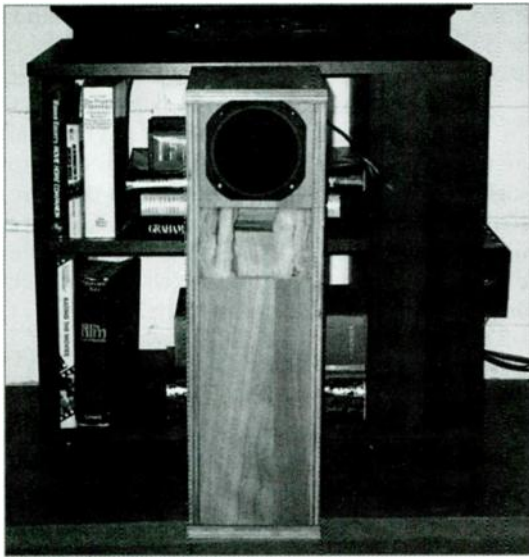
PHOTO 2: A third speaker using the newer fiberglass absorber arrangement. All three speakers have now been upgraded in this same way.
