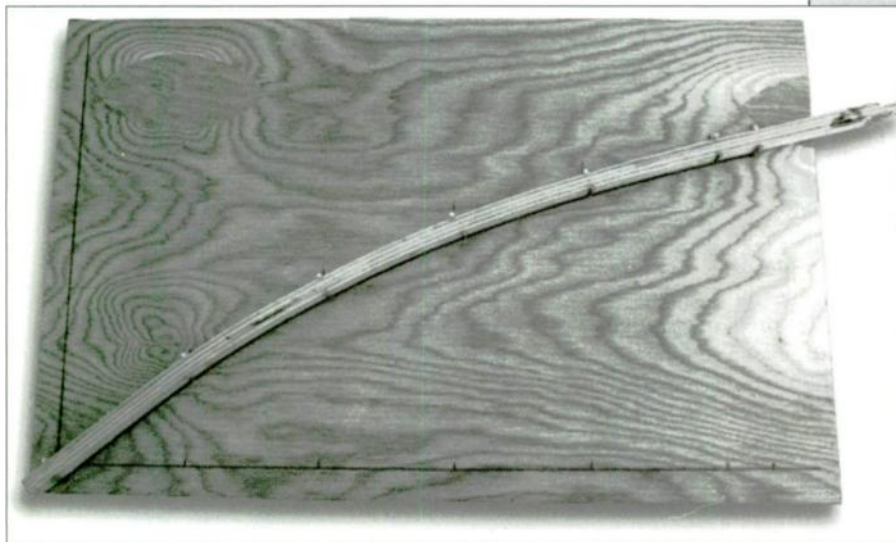
PHOTO 2: Forming the horn-brace and divider patterns.
