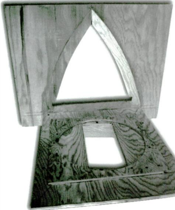
PHOTO 6: Baffle assembly attached to side with access-hole flange installed.
