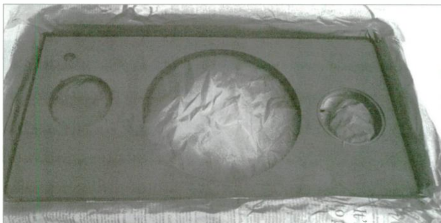
PHOTO 5: Baffle board sealed and painted.
