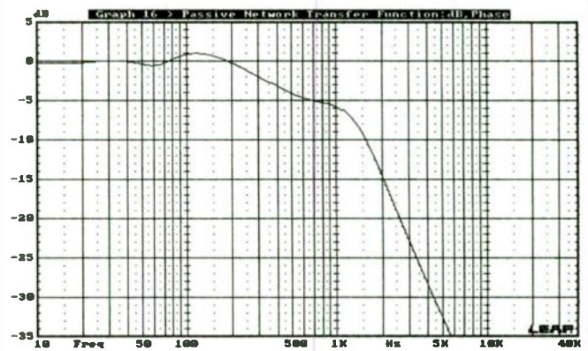
FIGURE 18: Simulated woofer crossover passive-network transfer function.
