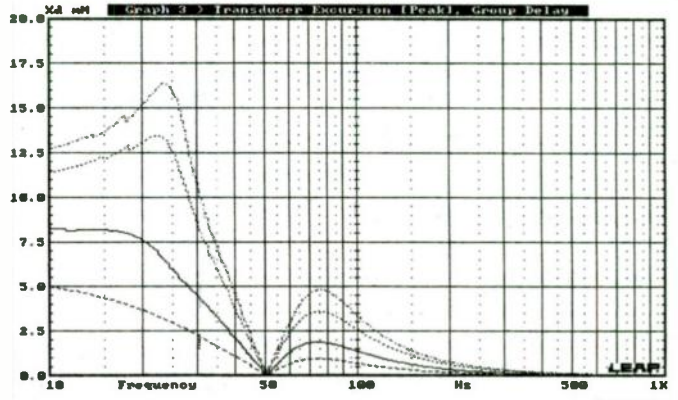
FIGURE 3: Simulation of driver-excursion curves for Fig. 2.
