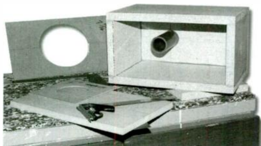
PHOTO 2: Masonite templates and partially completed enclosure.
