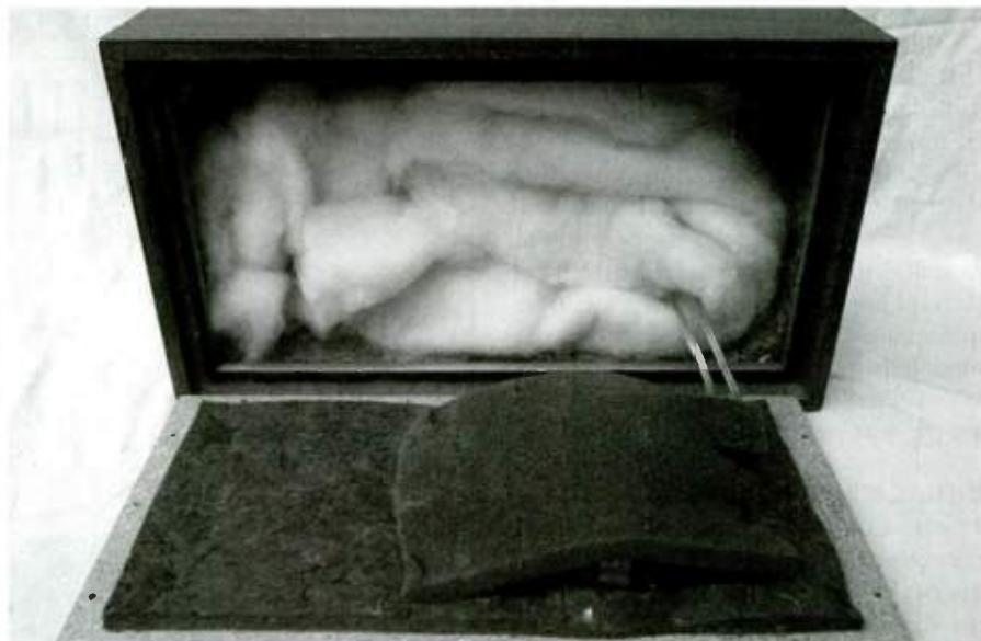
PHOTO 7: Sound-absorbing material installed.
