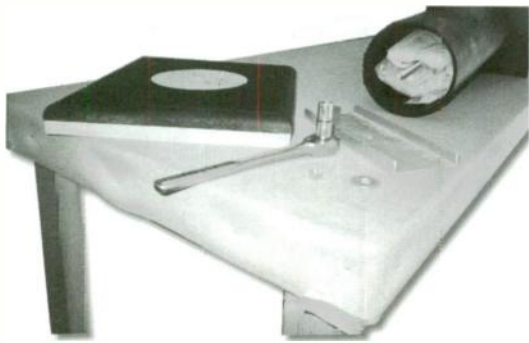
PHOTO 8: "The mortars"—steel pipe 6" in diameter with welded top plate matching cabinet base dimensions. 3/8" "all-thread" is bolted tight top to bottom. Aluminum channel is inverted under 1 3/4" bottom and torqued down. Note: sand weights are freezer bags taped closed to prevent sand from spilling in the event of poor assembly.
