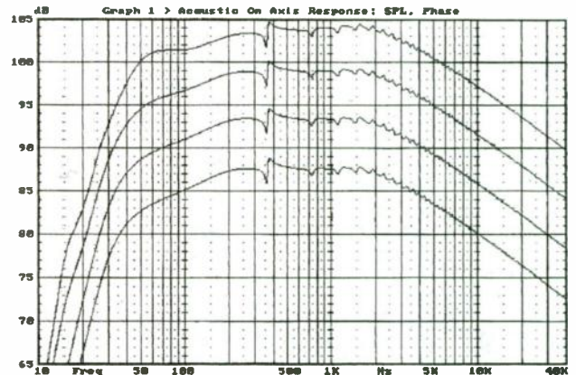
FIGURE 1: Low-frequency SPL simulation of the Vifa M22WR in the Woodstyle WS803 cabinet at 1, 4, 16, and 64W.
