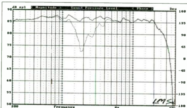
FIGURE 67: Comparison of system SPL with midbass and tweeter "hooked up" in-phase and reverse-phase.
