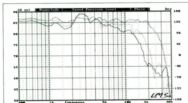
FIGURE 70: The satellite's measured on-axis SPL response compared to 30° and 45° horizontally off-axis.
