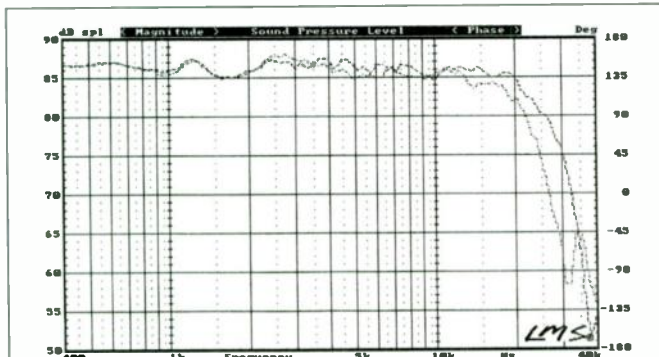
FIGURE 69: The satellite's measured on-axis SPL response compared to 15° horizontally off-axis.
