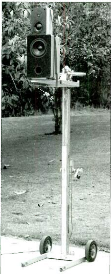
PHOTO 2: Subwoofer/satellite system on Load Jockey 350.
