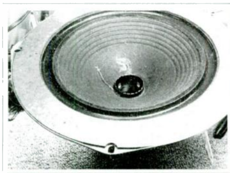
PHOTO 3: Insert glued in place. Also visible are the tabs bent in at the rim, and two of the four vent holes.
