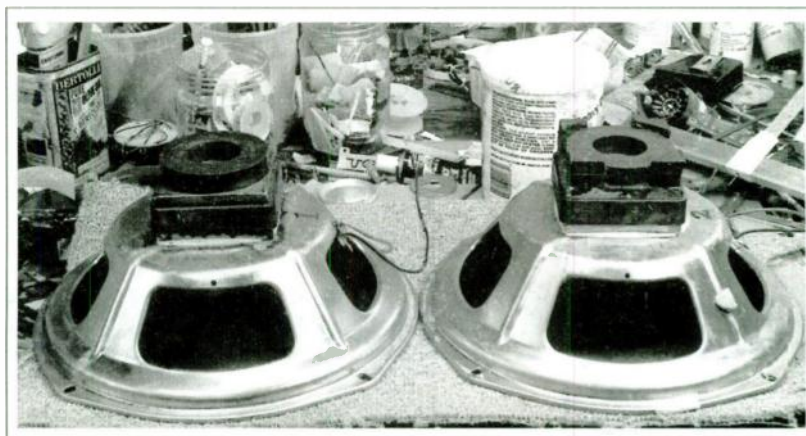
PHOTO 6: Backsides of the two woofers, complete except for the filters pasted over the frame cutouts. Note the more extensive bucking magnet coverage on the right, used to equalize motor strength. And you thought your workbench was cluttered?
