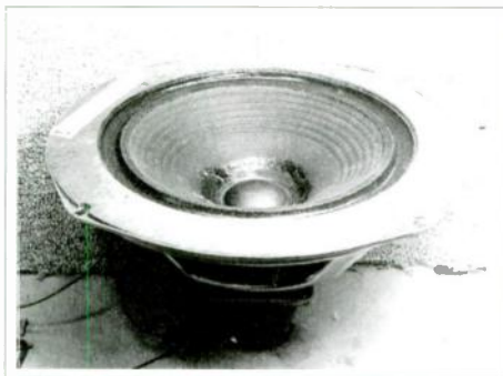
PHOTO 4: Structural modifications complete. The cone has a good coat of epoxy at the apex, and the hard, nonporous dust cap is securely glued, making for a much stiffened assembly.
