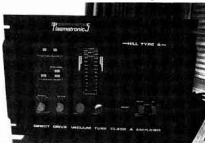
*The Plasmatronics direct-drive all-tube Class-A power amplifier.*
