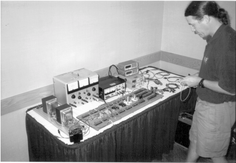
Grego Sanguinetti, getting ready to fire up the Universal Breadboard Amp. Over a couple of hours, Grego and Paul demoed bi and single 2A3, 300B, 45, 211, 845, 10, 801, 5V572, all sorts of cool tubes! Photo by Tom Vetromile
