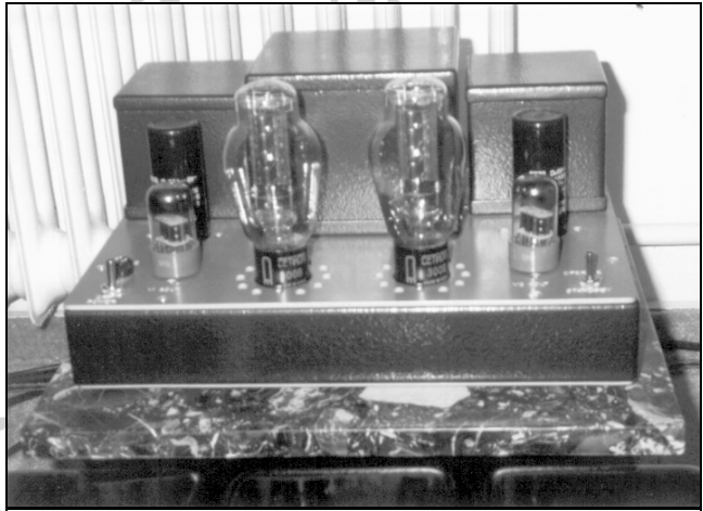
Rene's AES SE-1, in his custom built chassis with transformer enclosure. Rene' restores Porsche racecars for a living, and his skills make this a standout SE-1. Amp sports the signature mods.
