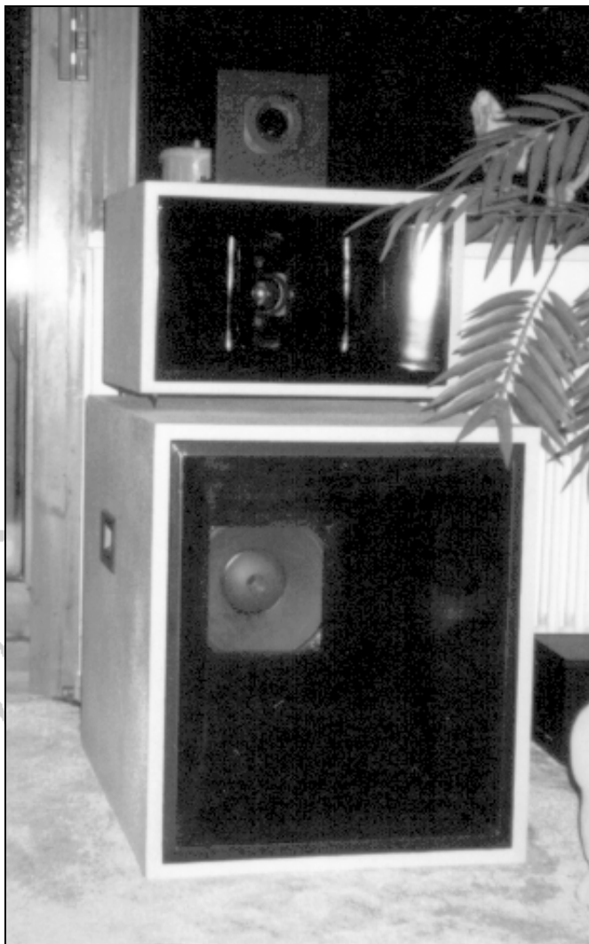
The original system, with Audax PR 120, Dynaudio D-54 in Edgarhorn style midrange horn, and Altec 414 in Edgar style 100Hz bass horn
