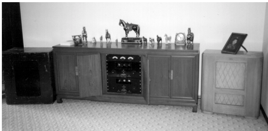
Crazy Eric's plan for vintage Xtasy - a pair of Western Electric 60A PP 205D amps and complementary WE meter panel, in a custom built mahogany console which hides the CD player and preamp. Speakers are 600 ohm Jensen coax units, in vintage Altec cabinets. Photo by Tom Vetromile.
