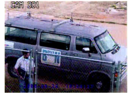
Photo 7. The pan-tilt-zoom camera can be used to verify site access alarms during normal hours. In this view a technician is accessing the site.
