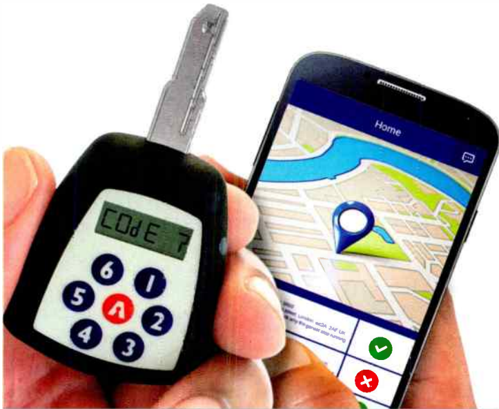
Photo 3. With a mechatronic lock, when the user arrives on site, verified by smartphone GPS, an access code is sent automatically that allows the key to open the lock to the site.
