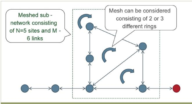
Figure 1. The network inside the green dotted box can be protected topologically. A single link failure will not affect any site;
