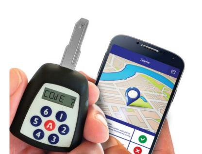
Photo 3. With a mechanatronic lock, when the user arrives on site, verified by smartphone GPS, an access code is sent automatically that allows the key to open the lock to the site.
