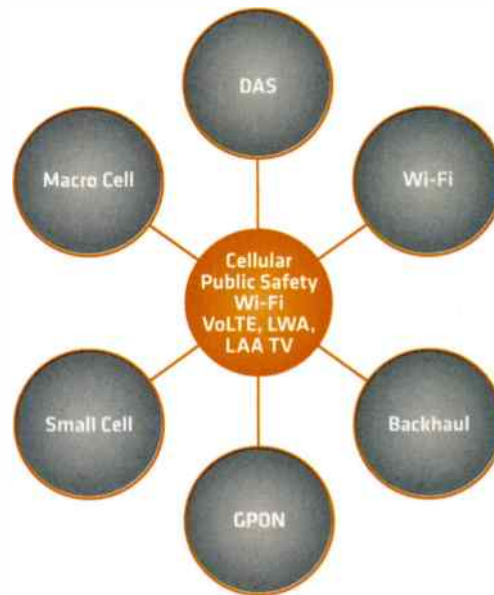
Figure 1. With convergence, an integrated system can support the operation of multiple services including cellular, public safety, Wi-Fi, VoIP and IPTV over the same infrastructure.
