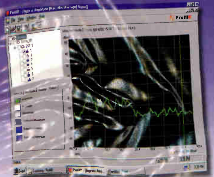
TrafficControl™ measures and plots ingress spectrum of bands fully occupied by return traffic
