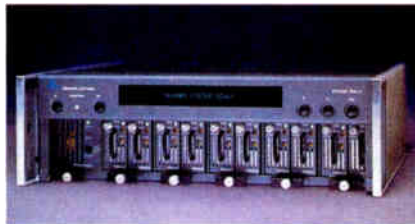
The industry's most cost-effective, compact 1,310 nm distributed feedback (DFB) transmitter
