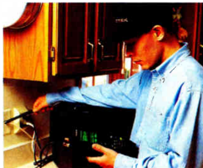
The Home Wiring Test System helps verify the quality of a cable installation.
