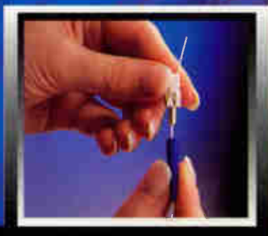
Step 2: Prepare the cable by sliding the stair-step boot, small end first, down the "field" fiber until it is out of the way. Next, slide the pre-assembled crimp body inner housing assembly, small end first, down the fiber.
