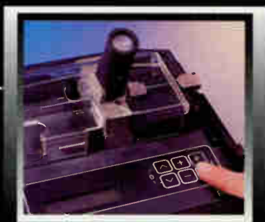
Step 6: To fuse the "field" fiber to the ferrule, close the splicer cover and clean the fiber with a brief arc. Following the prompt, fuse the fibers.
