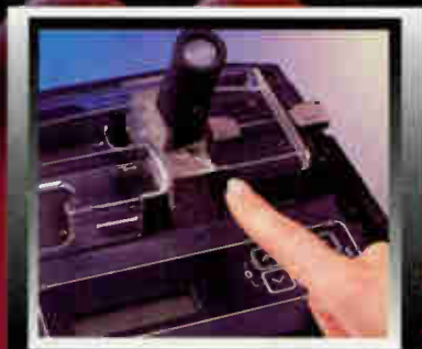
Step 7: Crimp the lead-in tube around the buffered fiber by pressing down firmly on the crimp lever.
