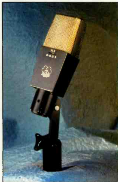
The AKG C414B has a four-position switchable polar pattern.
