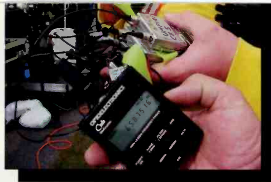
To verify usage, a variety of tools are used by the coordinators, such as this portable frequency counter.
