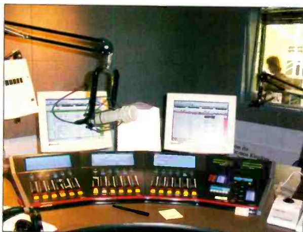
The Epicenter is designed to operate with third-party controllers like the Logitek NuMix.
