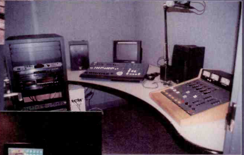
The Heart of the Facility: The staff and students of WMCX-FM are delighted with their new On-Air/Master Control Room with Harris' AirWave Digital 20 on-air console and Scott Studio LCD monitors.
