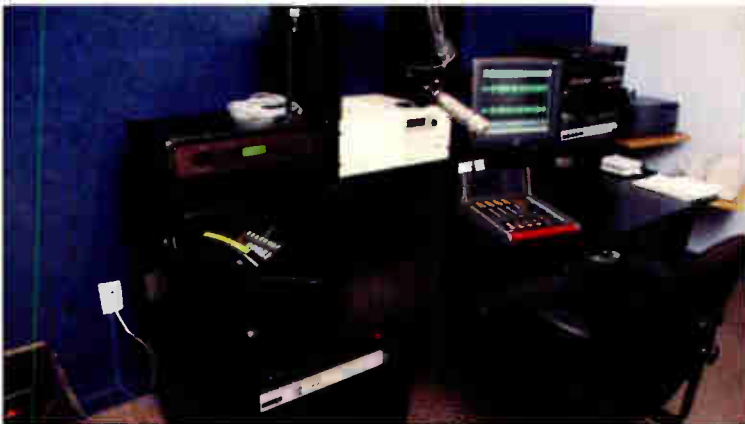
The production studio is the smallest studio. The console, which sits on the tabletop and is connected by a few cables, can be placed wherever it is needed when the room is in use.
