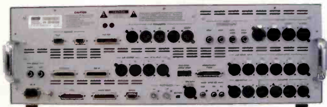
The console's audio, control and data connections are on the back panel.
