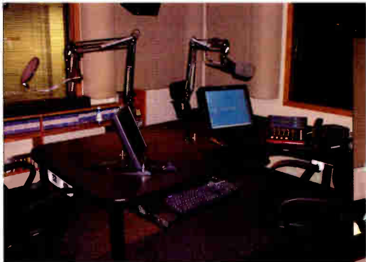
The production studios have small consoles because all the signal manipulation and mixdown is done in the DAW software.
