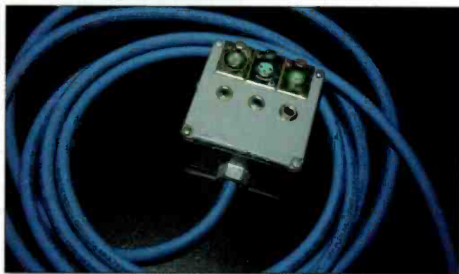
The homemade snake uses a PVC electrical box.
