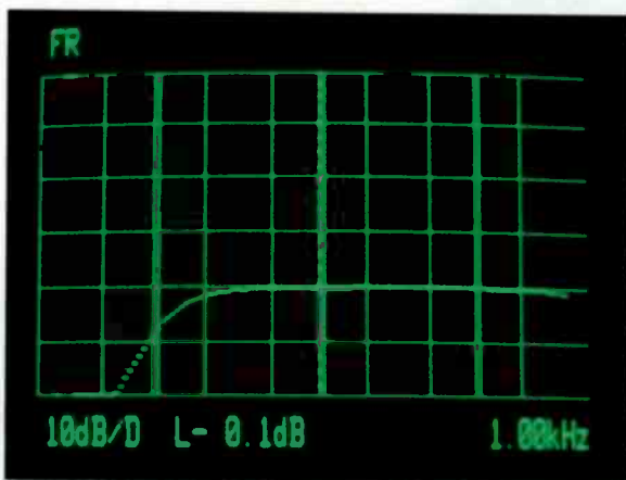
Figure 1. The response with all the bands disabled and the low frequency roll-off filter set to 150Hz.
