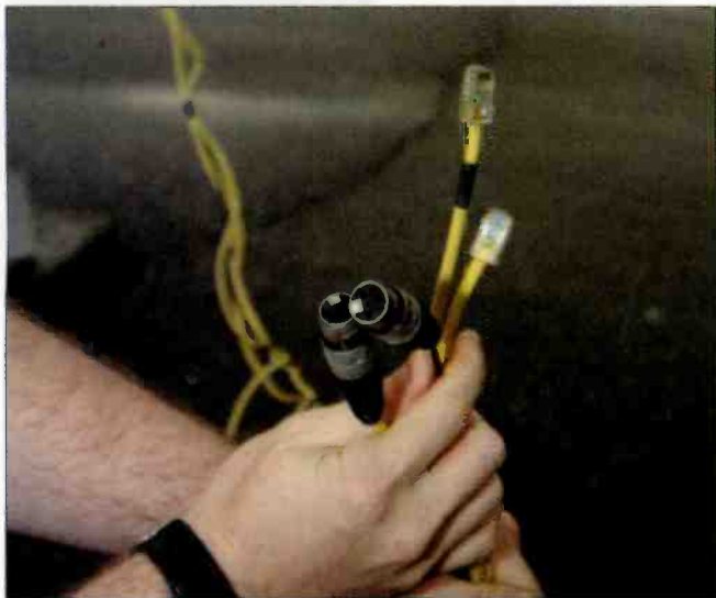
The flying snake uses CAT-5 cable and a run of Belden 9451.
