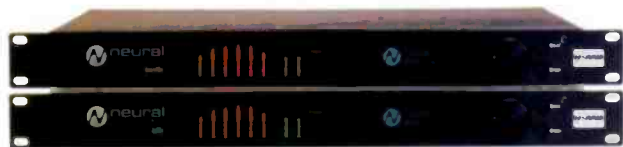
The Neural Downmix (top) and Upmix were used to encode and monitor the surround material for stereo transmission.
