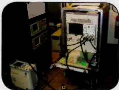
The test equipment setup that was used to sweep the antenna.
