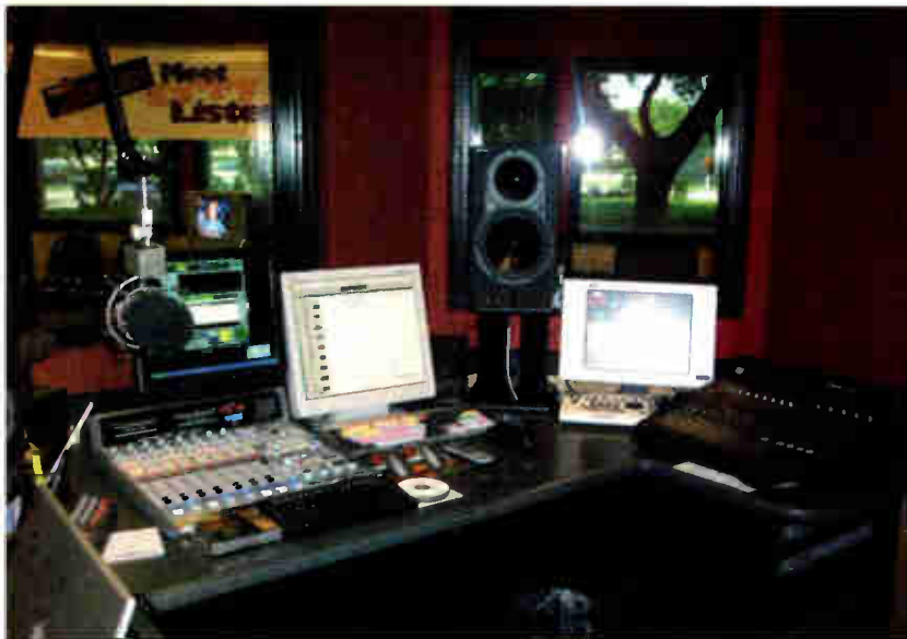
Another view of Production 1 with the Wheatstone G-6, Audio Vault AVRPS screen and Pro Tools HD system centered for the operator's convenience.
