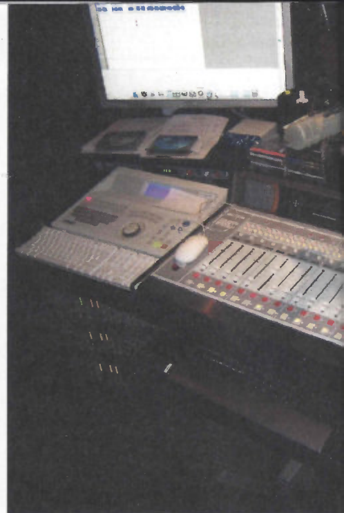
The morning show control room has a profanity delay, behind the Short Cut, with a red dump button visible on the console surface.
