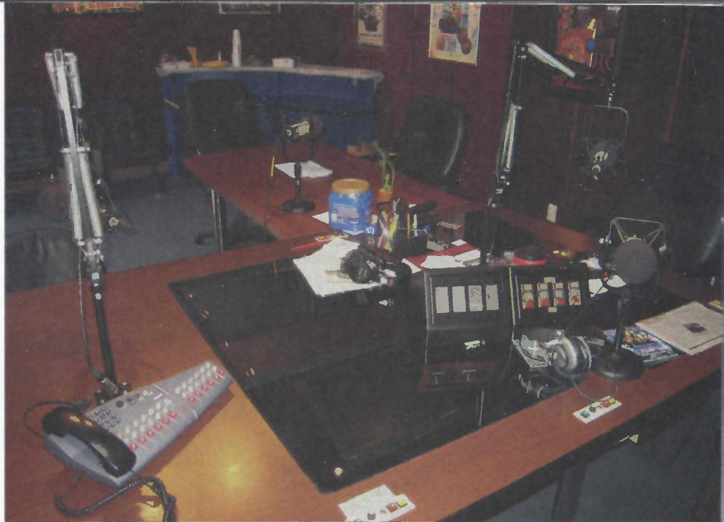
The talk studio provides plenty of control for the host including all mic on/off/cough, phone speaker and monitor levels, phone system, and a view of the Media Touch screen.
