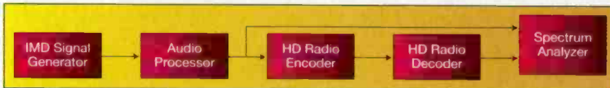
Figure 1. The test setup used to analyze low bit-rate audio.
